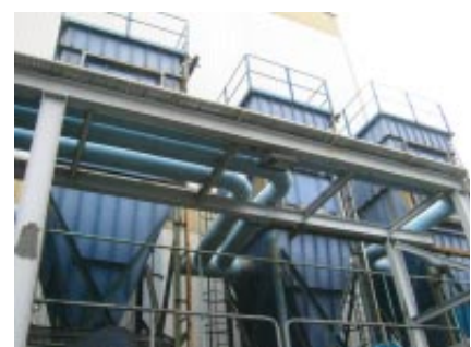
Example of a bag filter in a factory
