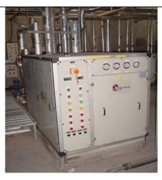
Water scrubbers are used in paint grinding workshops to reduce the amount of inhalable particles released to the environment.
